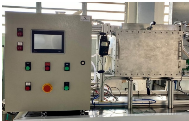
Figure 1. Prototype for batch process in the microwave oven.
